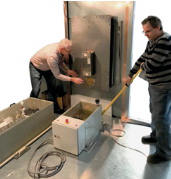
E1/E2 test conductive (N)EMP test filter
