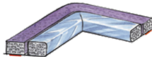
Figure 26.2: A EMI gasket combined with an environmental seal.
