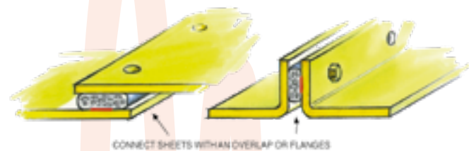
Figure 26.1: Examples of a stiff construction to prevent openings.
