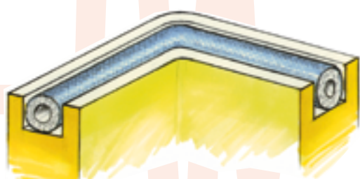
Figure 41: Groove construction with conductive o-ring gasket
