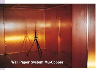
We produce Faraday cages, shielded chambers and other shielding components like:
