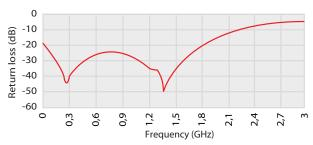
3 mm thick ferrite tile + 21 mm gab + 3 mm thick ferrite tile
